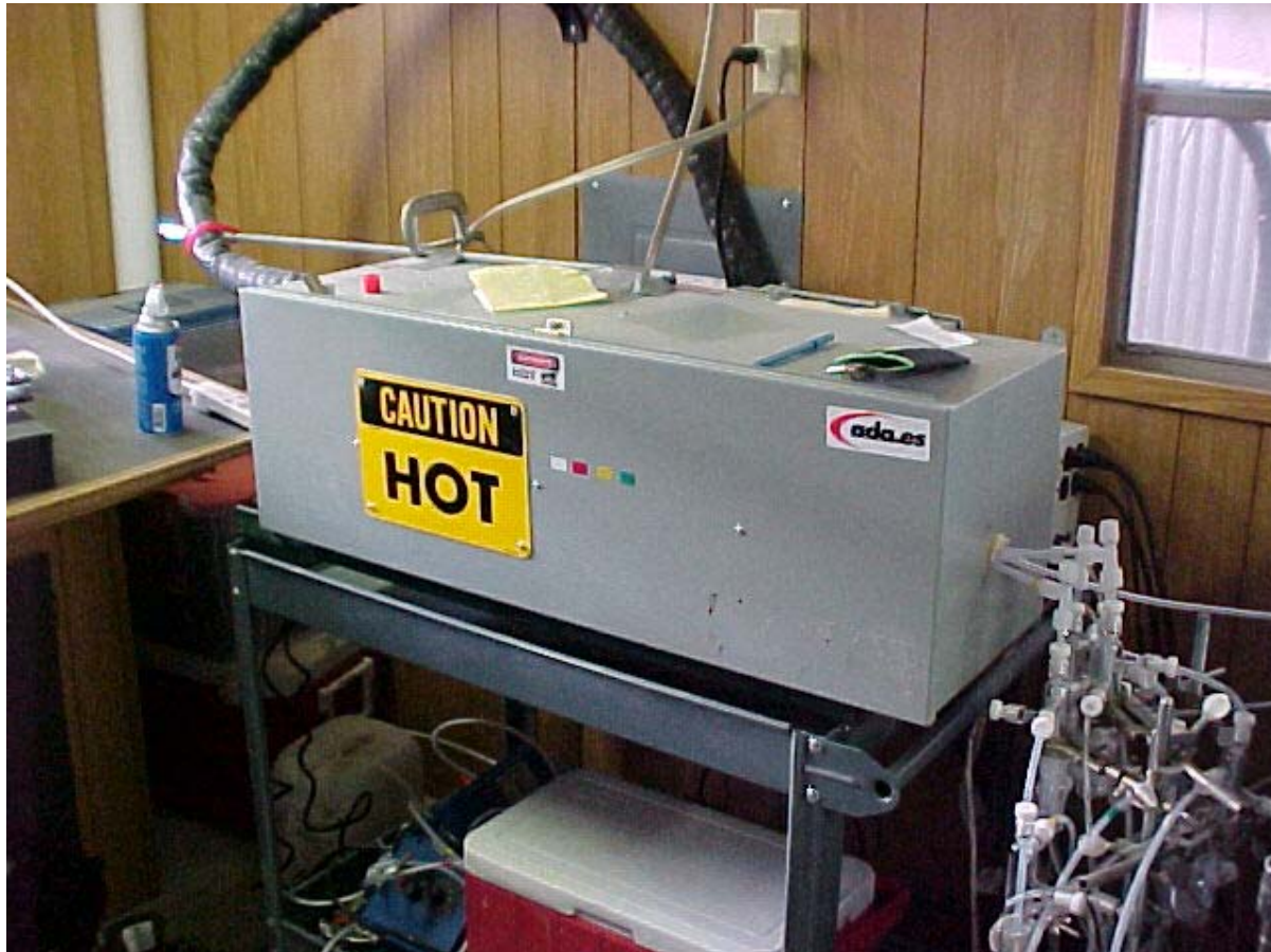
Figure 2. Sorbent Screening Device—Heated Box and Impingers.
